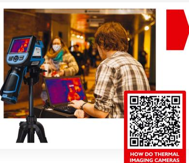
Well, I can use an infrared thermometer or a thermal image camera suitable for that application ensuring I use them the right way. The contactless measurement of a body's surface temperature is performed by detecting its radiated heat. It is available from PROMAX a comprehensibe explanation on how do these devices work by scanning the QR or opening this link:
